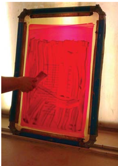
Proper ink management prior to cleaning
