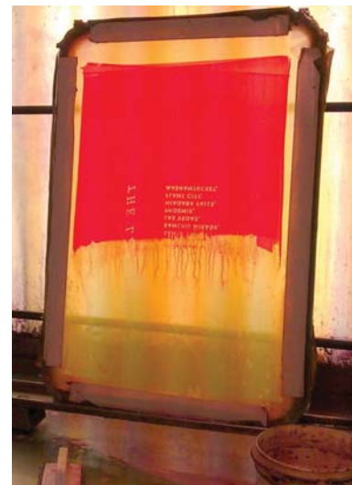
Emulsion removed from half of the screen
